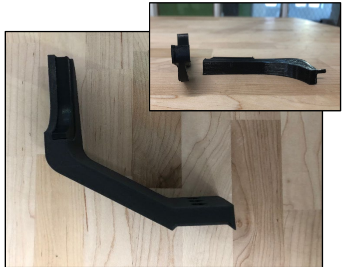
Figure 2: The two-part EOAT consisted of a rigid backbone for strength [bottom left] and a flexible piece that would conform to the workpiece [top right].
