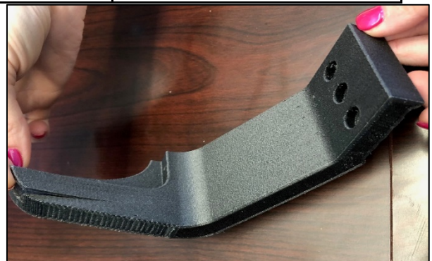
Figure 7: Design tolerances were adjusted for assembly due to cracking in the dovetail joint of the original rigid arm.
